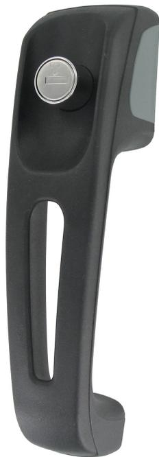
This handle was specifically designed for off-highway vehicle applications that require a surface mounted exterior push button handle with 163mm mounting pattern. It is retrofittable with most European push button handles and offers robust construction, ergonomic function and styling for a very cost effective price.
